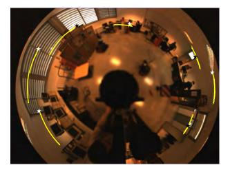
Fig. 12. Some of the tracked points (stars) and their motion in the image along a sequence.
